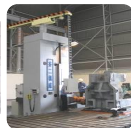
Boring(Floor type) M/C
