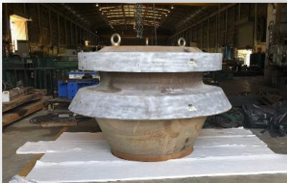
Roller Boss repair
