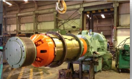
Mandrel Down coiler Overhaul and repair
