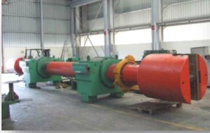
Main drive spindle Overhaul
