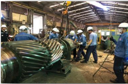
Pinion Shaft Overhaul
