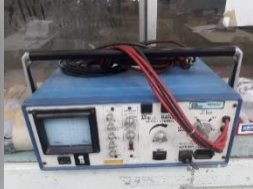
6.6KV Surge Comparison Test
