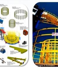
Turntable Capacity Turntable Dimension Rotation Speed Hydraulic Motors Maxinum torque Maxinum pressure Power Hydraulic Pumps Flow per motor Working Pressure Shaft Power Electric Motor Mechanical Drive Total Weight : 5,000 Tons : Ø 25.0 m., High 10.2 m. Max. 0.4 RPM : 4 (3+1) Unit : 49,000 Nm./Motor : 350 bar : 75 KW. : 2 Unit : 330 LPM : 310 bar : 93 Kw. : 160 Kw. 380 V. 4 Pole x 2 : Chain and Sprocket : 520 Tons.
